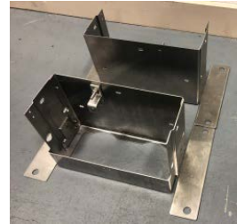
Dual Pad Mount Brackets (2 holes in mounting feet)
